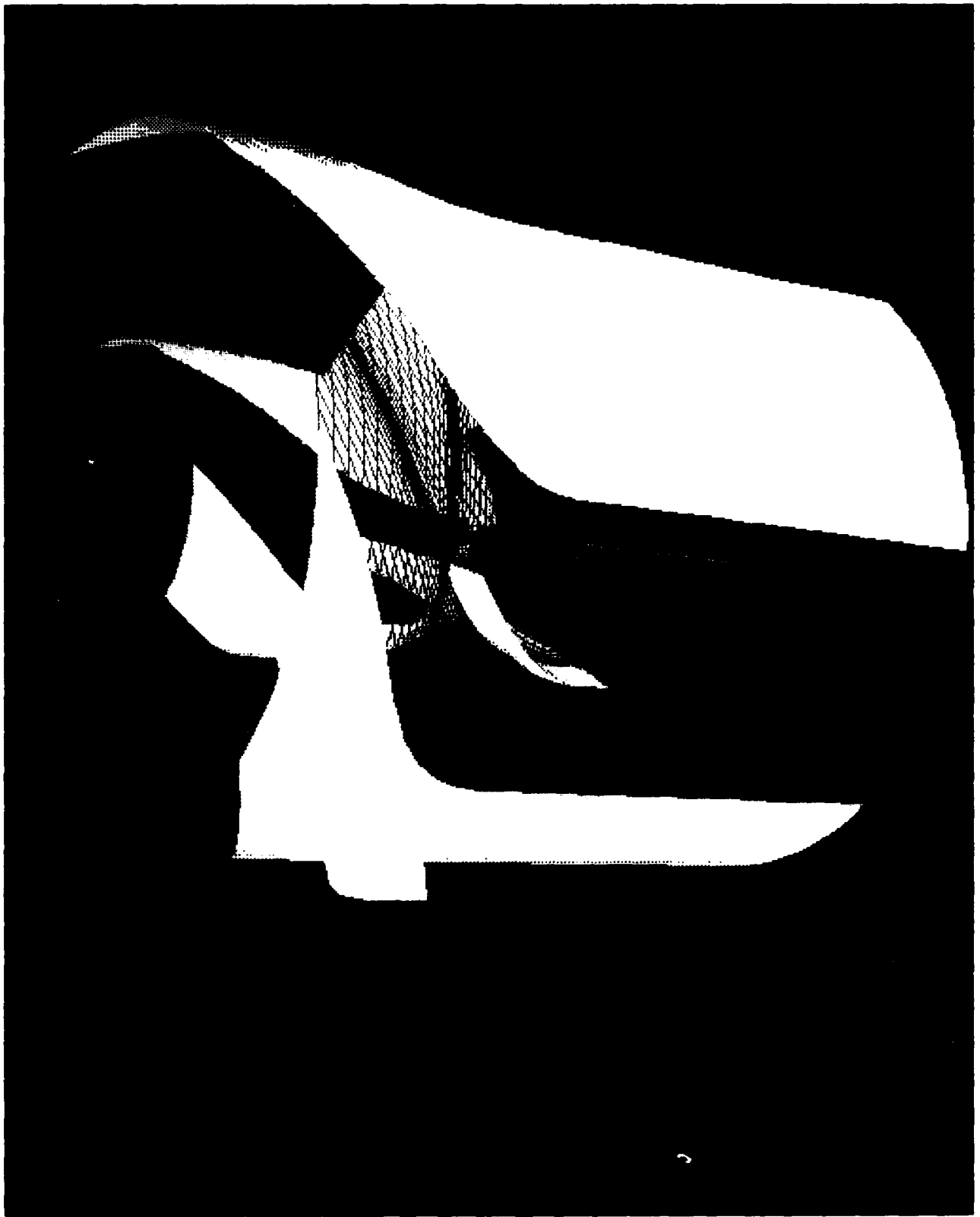
Figure 6. Hub and Shroud Coordinate Surfaces with Three Blades.
