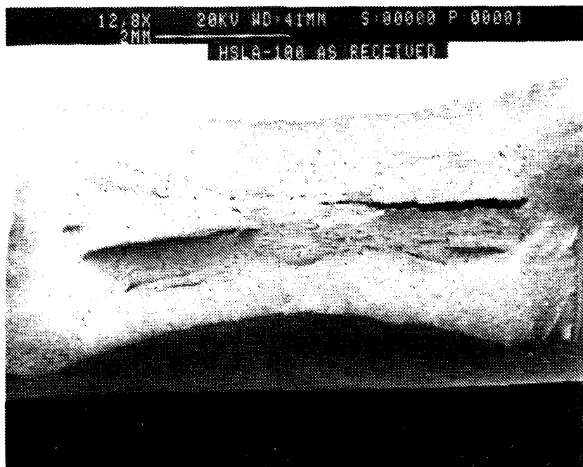
Figure 38. SEM Low Magnification Fracture Surface of Flat Specimens, Fractured at Room Temperature in the Base Metal
