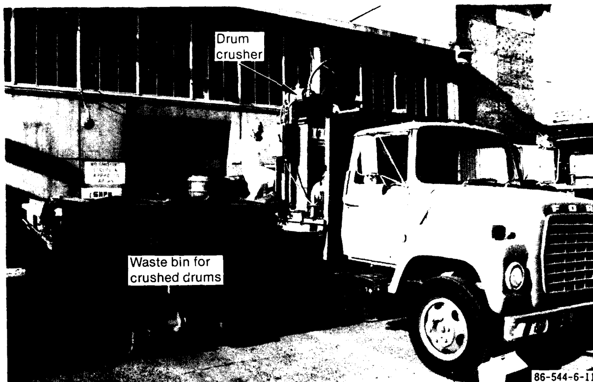
Figure 27. Truck-mounted drum crusher. A waste bin is on the left.
