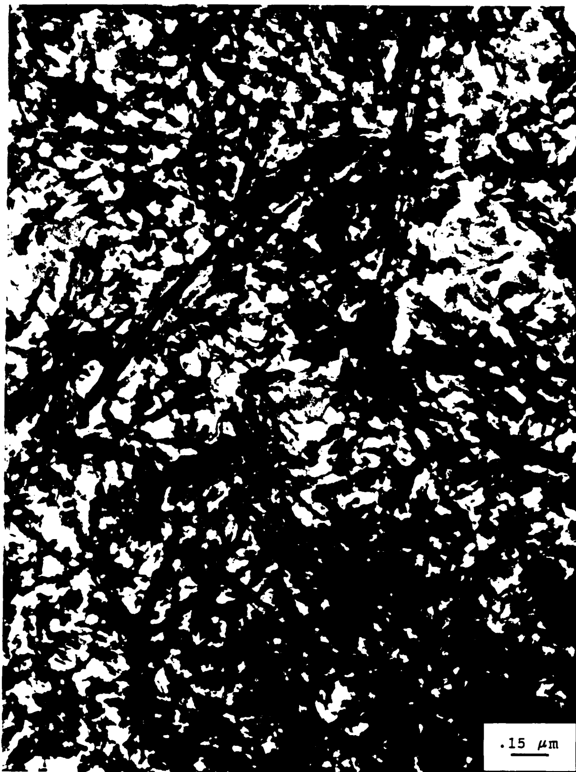
Figure 12. TEM micrograph containing anisotropic AlN fibers surrounded by a BN matrix.
