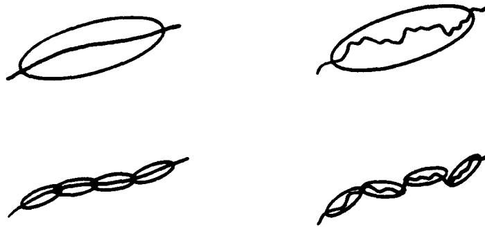
Figure 4.15: At coarse scales a long smooth edge and a long jagged edge appear identical. Only at finer scales do edge primitives obtain sufficient resolution to distinguish smaller scale detail.
