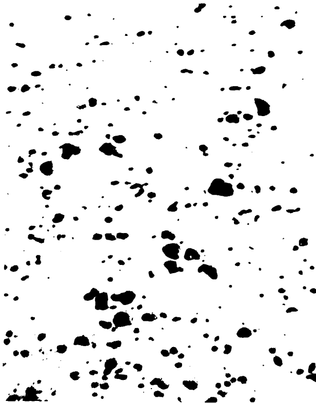
Figure A3-3. Cavitation in Supral 220-T6 at location M2
