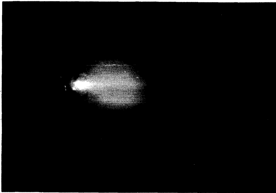
Fig. 3.4 Hollow Cathode Ignited mode Configuration
