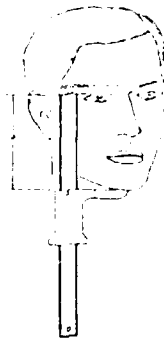
Figure 10. Measuring face length with the sizing caliper.
