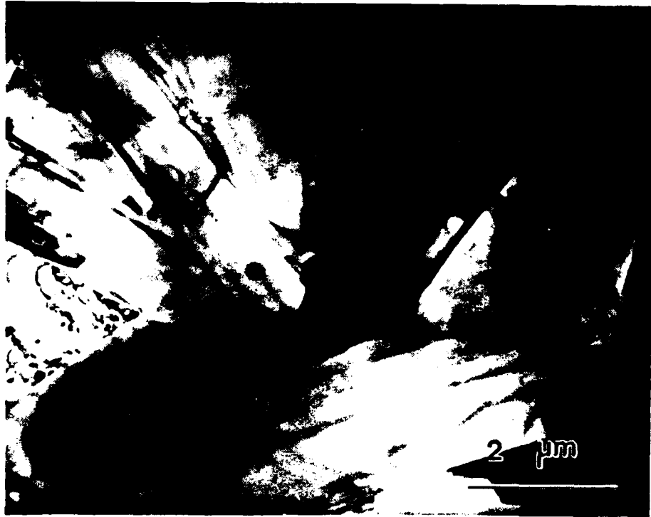
Figure 27 TEM micrograph of 37Y2 after annealing at 1860°C for 48 hr, showing a lot of elongated grains
