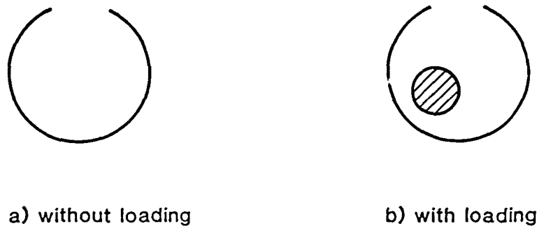
Fig. 2 Slitted cylinder cavity (a) without loading (b) with loading.
