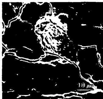
Fig. 2. Scanning electron micrograph of a CZ matrix containing a \gamma -C 2 S particle transformed during grinding and polishing. Extensive microcracking occurred in the surrounding areas.
