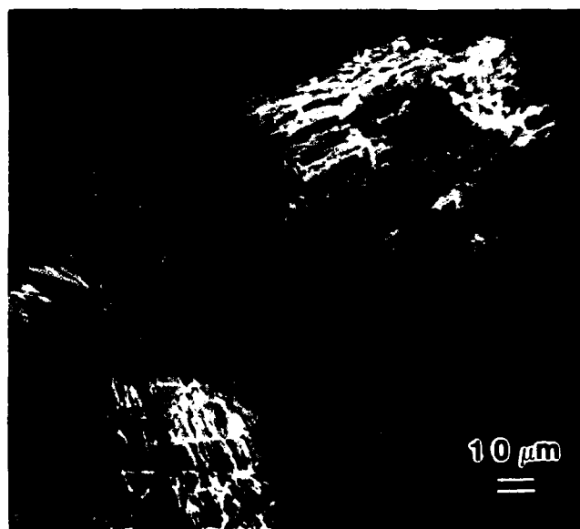
Fig. 8. SEM micrograph of C 2 S grains which underwent \beta \rightarrow \gamma transformation and "dusted" because of the accompanying large 12% molar volume increase. 24
