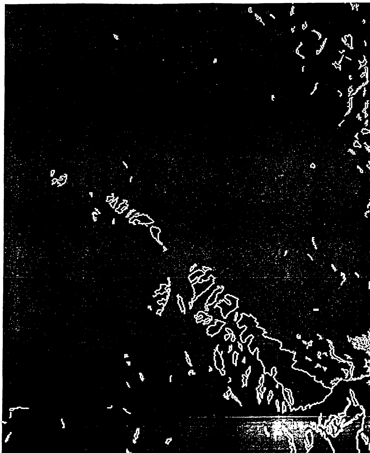
Vectorized Shadow Boundaries of SAR Image, Brzeau Range Area Minimum contour length: 10 pixels Threshold for shadow boundaries: 43
