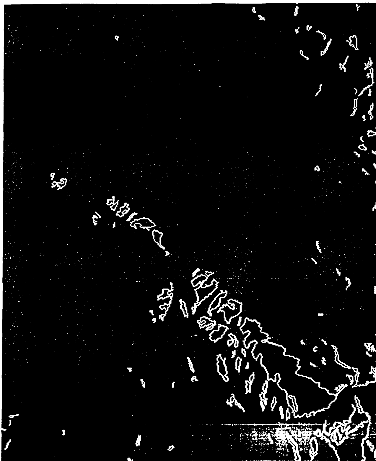
Vectorized Shadow Boundaries of SAR image, Bransau Range Area Minimum contour length: 10 pixels Threshold for noise removal: 13
