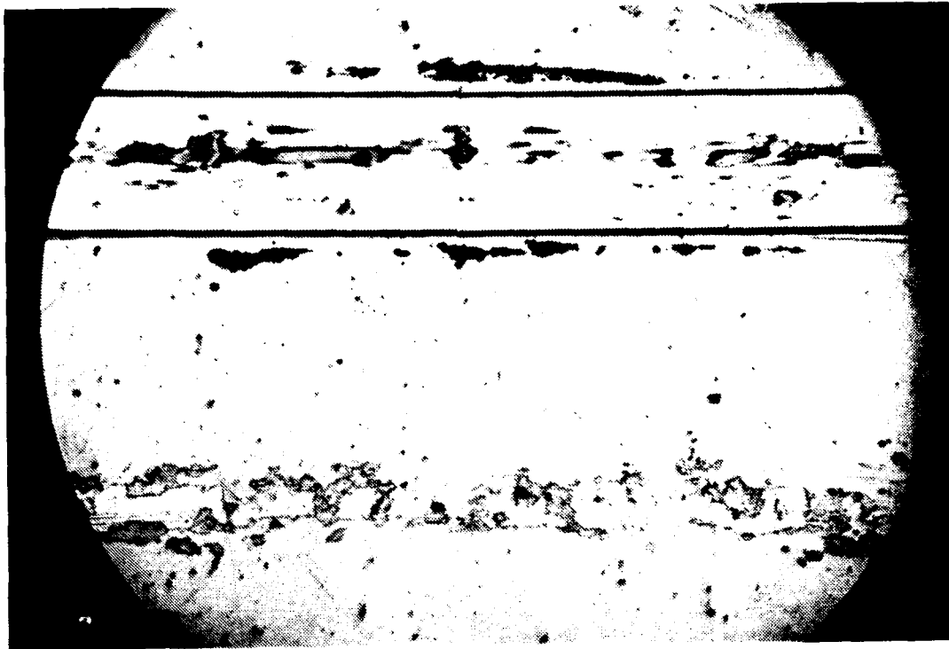
Figure 23. Wear Groove in 52100 Steel Disk. Top track is Silicon Nitride ball sliding in dry Nitrogen atmosphere. Bottom track is Silicon Nitride ball sliding in air.
