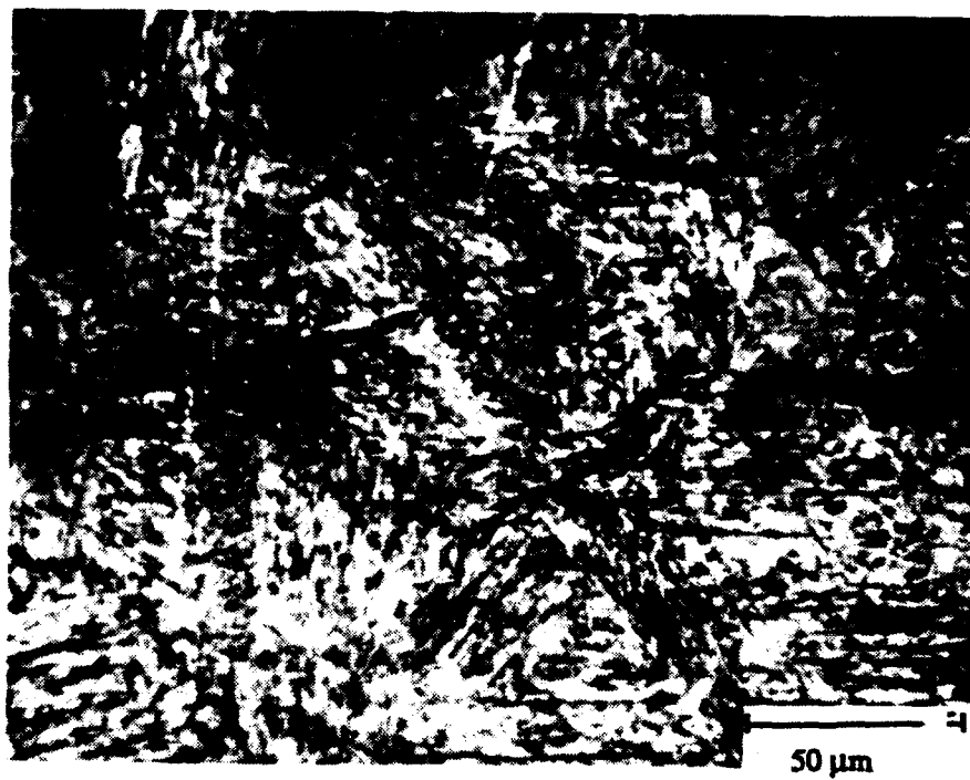
Figure 3.10: 4140 Heat-Affected Zone Surface Microstructure.
