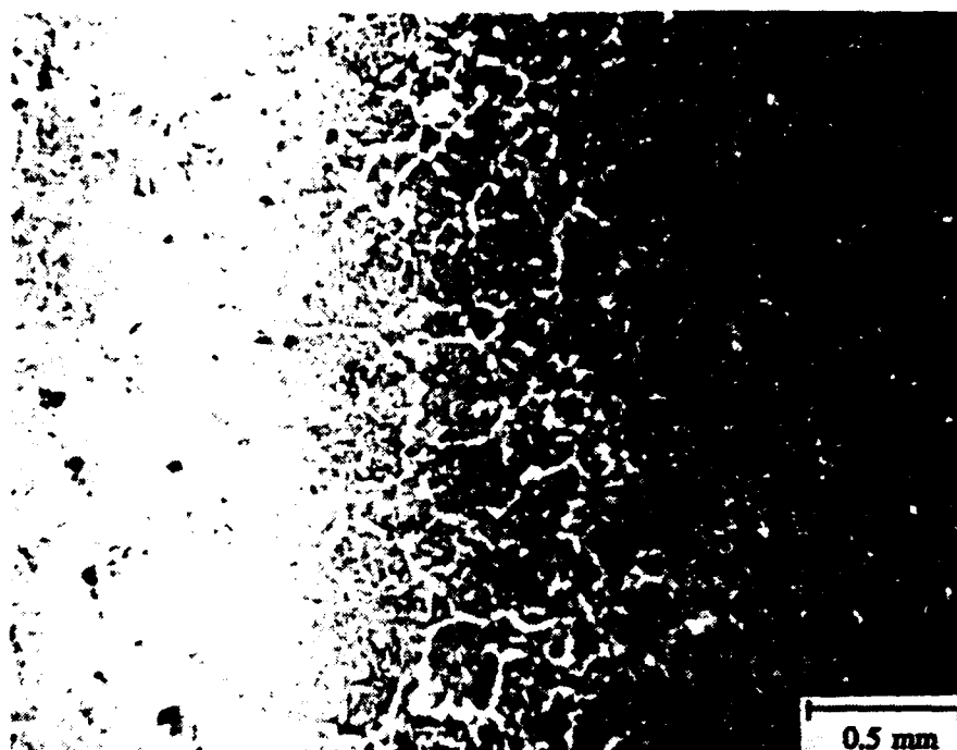
Figure 3.3: Section of Top Surface of Weldment Showing Regions from HTS (Left) to HTS Heat-Affected Zone (Near) (Right).
