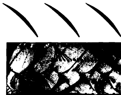
Fig.43 Cascade section and Schlieren picture of 30° camber DCA blade at sonic inlet velocity
