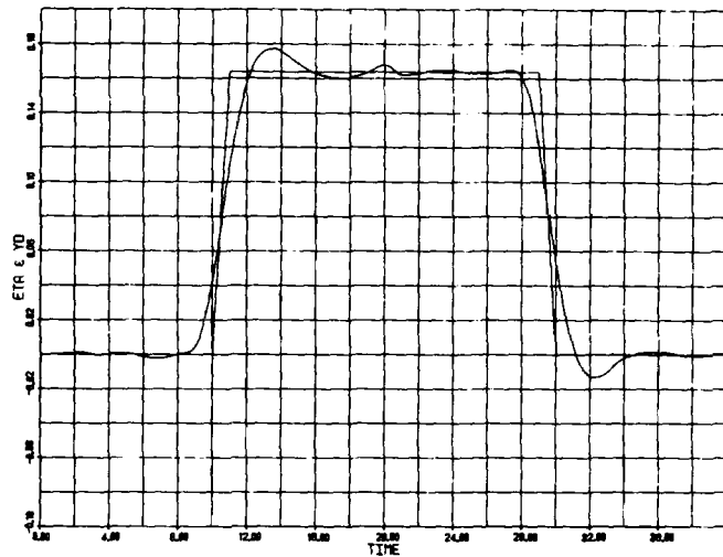
Figure 9. Desired and Actual Ship Path in Passing in a Channel
