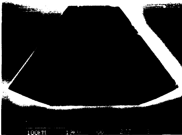
Figure 4. Cross section of a beam obtained with a double sided etch in EPW. No \{110\} planes are visible in this case because of their low etch rate compare to the \{311\} in this etchant.
