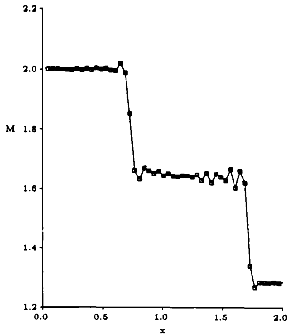
Figure 13: Mid-channel Mach Number, M_\infty = 2 , 10 Degree Wedge, Galerkin Method
