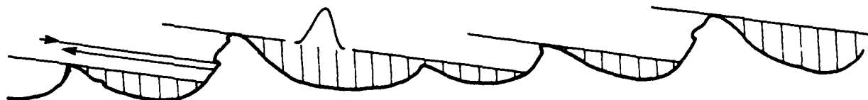
FIGURE 15. The geometry for upwind radar illumination from a shipboard radar is shown, wind and waves moving right to left. Wave breaking occurs on the leeward face, and sheltering of this face by steep waves is expected as described in the text.
