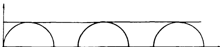
Figure 4. Failure envelope for saturated, purely cohesive sediment.
