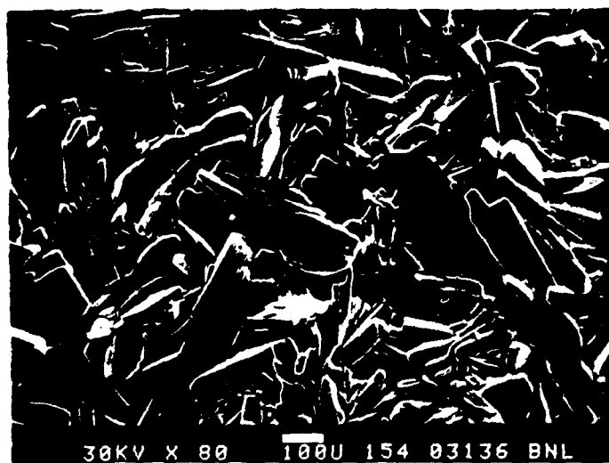
Figure 3. Photomicrographs of p(AMSA), p(AM) and p(VP)-modified Zn·Ph crystal surfaces which suggest that no significant changes in the crystal size occur.
