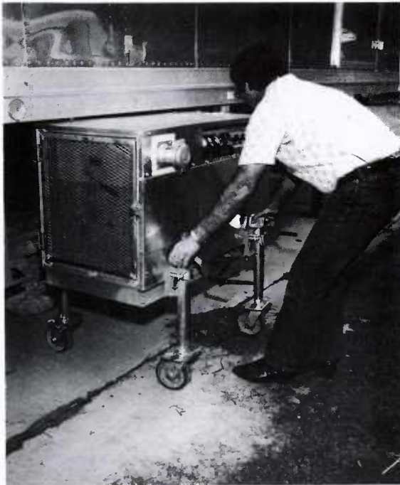
Figure 6. Photographs of one of the two diesel-powered alternators while still fixed to the MFL undercarriage (top left); in the process of lowering and adjusting its wheel-type support legs (top right); its removal from the undercarriage (bottom left); and its final setup for operation (bottom right).
