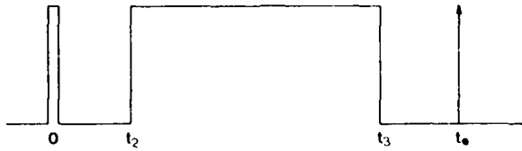
FIG. 6. Excitation pulse sequence of extended-pulse photon echo (EPPE). The maximum echo signal occurs at t_e = t_3 + t_2 - t_1 , denoted by the arrow.
