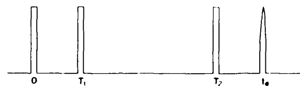
FIG. 4. Excitation pulse sequence of conventional three-pulse photon echo (SPE). The echo is emitted at t_e = T_1 + T_2 .
