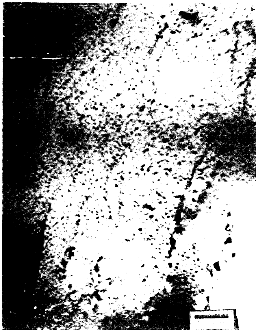
Figure 16 Apparent dislocation-particle interaction in under-aged binary alloy. Note apparent shearing of particles.
