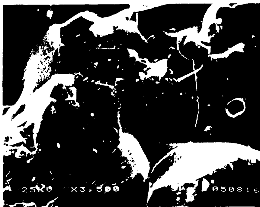
Figure 15, Transgranular fracture crossing several grains; velocity = 12.5 m/s.
