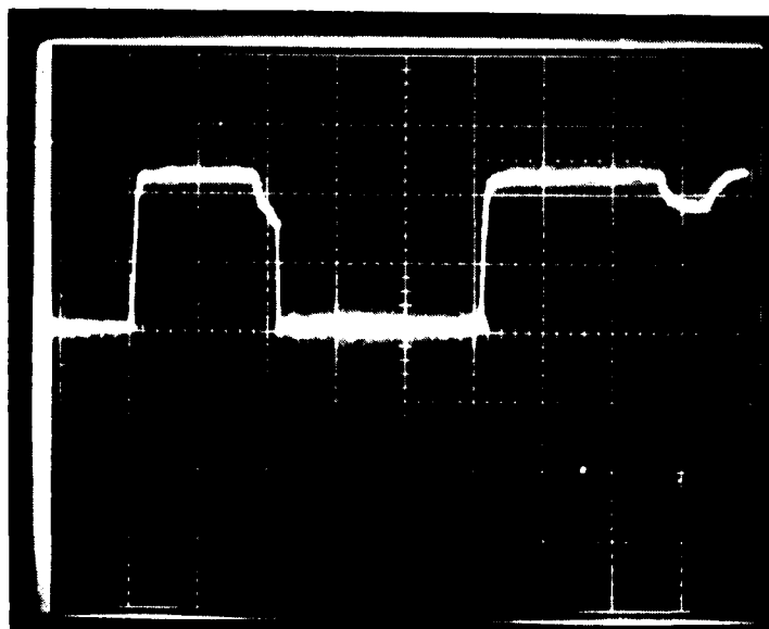
Figure 68. 51-ohm resistor, 1 \mu s/div, 2V/div.
