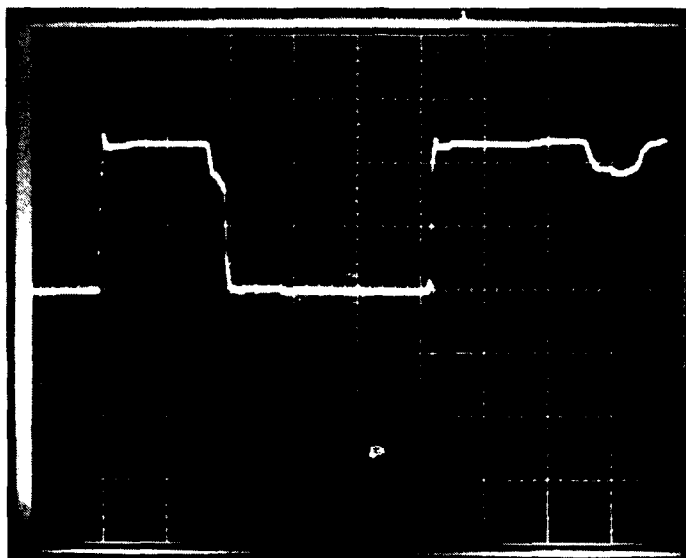
Figure 72. Primary power plane with 51-ohm termination, 1 \mu s/div, 2V/div.
