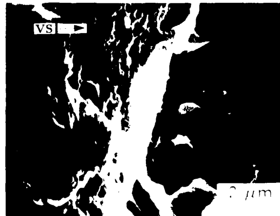
Fig. 10. High magnification view of an area containing fine dimples in a low temperature specimen (shot 85-15).
