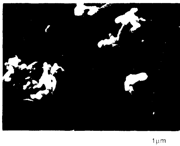
FIG. 6.6. SHORT TIME DEPOSITION SHOWING UNIFORM BACKGROUND LAYER ON A SAPPHIRE SUBSTRATE (30 °C, 1.3 TORR PARTIAL PRESSURE, 5 MINS)
