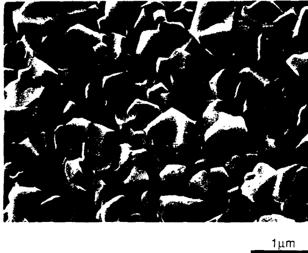
FIG. 5.12. SURFACE MORPHOLOGY OF A CADMIUM TELLURIDE LAYER DEPOSITED ON A GALLIUM ARSENIDE SUBSTRATE AT 250°C WITH \text{DMCd:DETe}=1.5 AND FOCUSED UV.
