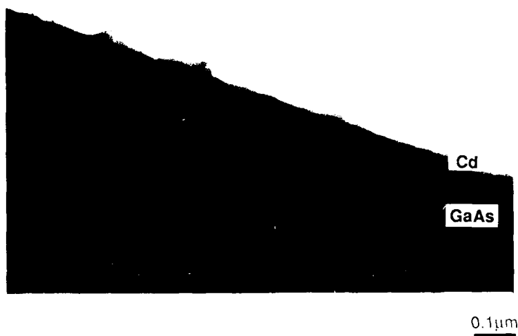
FIG 6.16. CROSS-SECTIONAL TEM MICROGRAPH OF CADMIUM DEPOSITED ON A GALLIUM ARSENIDE SUBSTRATE (0°C, 1.3 TORR PARTIAL PRESSURE, 60 MINS)
