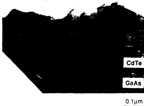
FIG. 5.13. CROSS-SECTIONAL TEM MICROGRAPH OF A CADMIUM TELLURIDE LAYER DEPOSITED ON A GALLIUM ARSENIDE SUBSTRATE AT 250°C WITH \text{DMCd:DETe}=1.5 AND FOCUSED UV.
