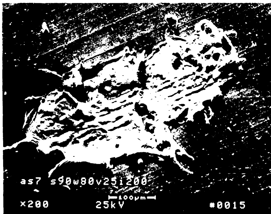
Figure 13. SEM micrograph of arc-sprayed zinc droplets showing shrinkage and conformation to substrate topography.
