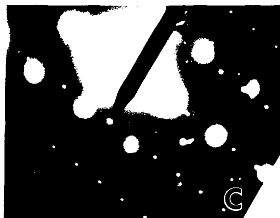
Figure 32. Grain Boundary Precipitate, Nb-1.2Ti-0.6N, Aged at 1200°C/4 hr
