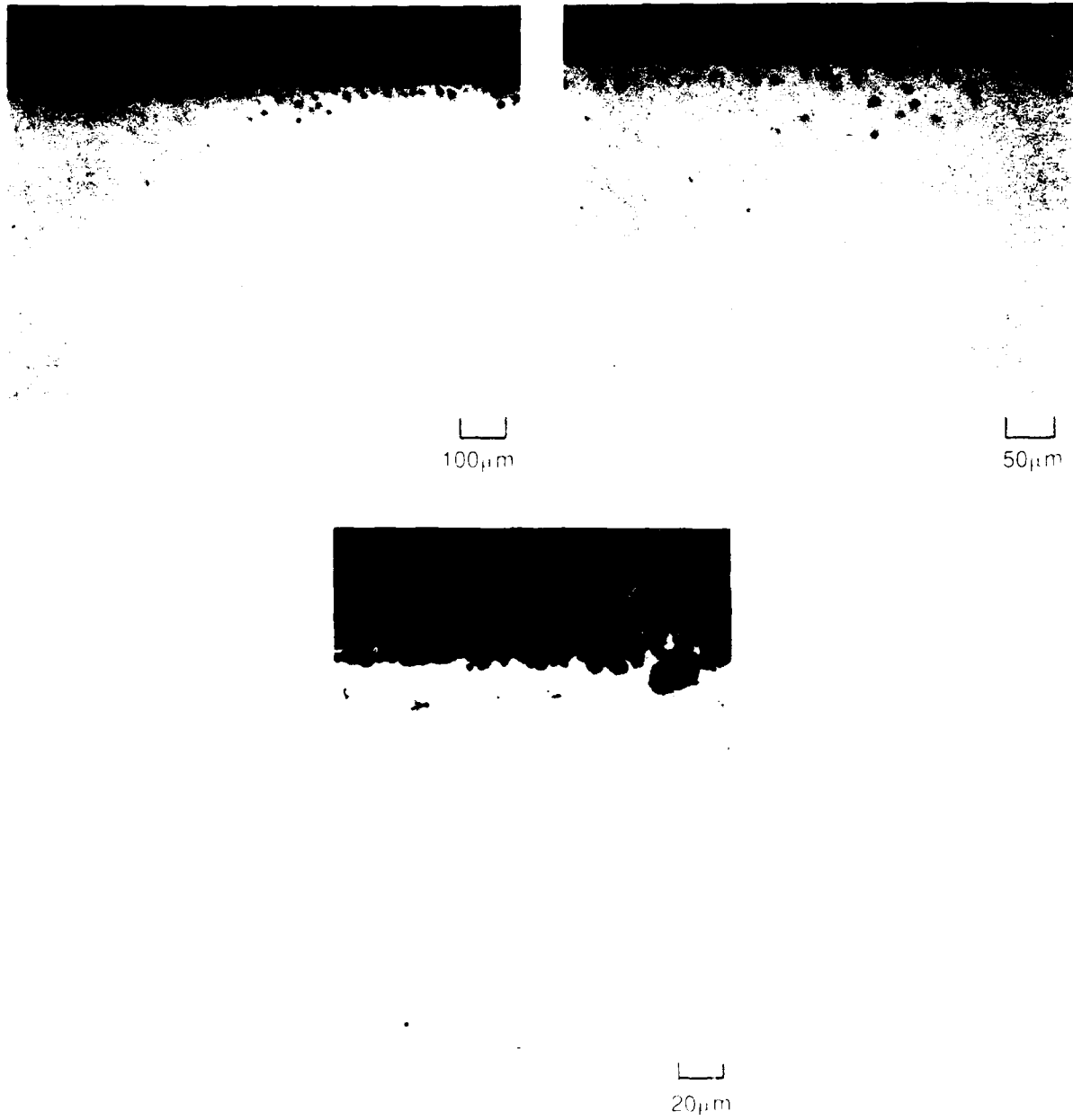
Fig. 8 High purity (low sulfur) Ni-40 wt % Cr cyclically oxidized to 1000°C in 0.1% SO 2 -O 2 for 1016 cycles. Optical micrographs.
