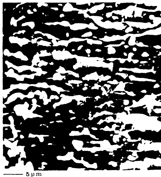
Fig. 3 SEM image of Sn/Sb oxide catalyst reduced in H_2 , indicating surface segregation of species
