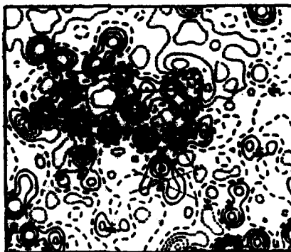
Fig. 1 : X-N difference Fourier synthesis of UHAF 50 Na, cut through molecular plane, contour interval 0.1 e/Å
