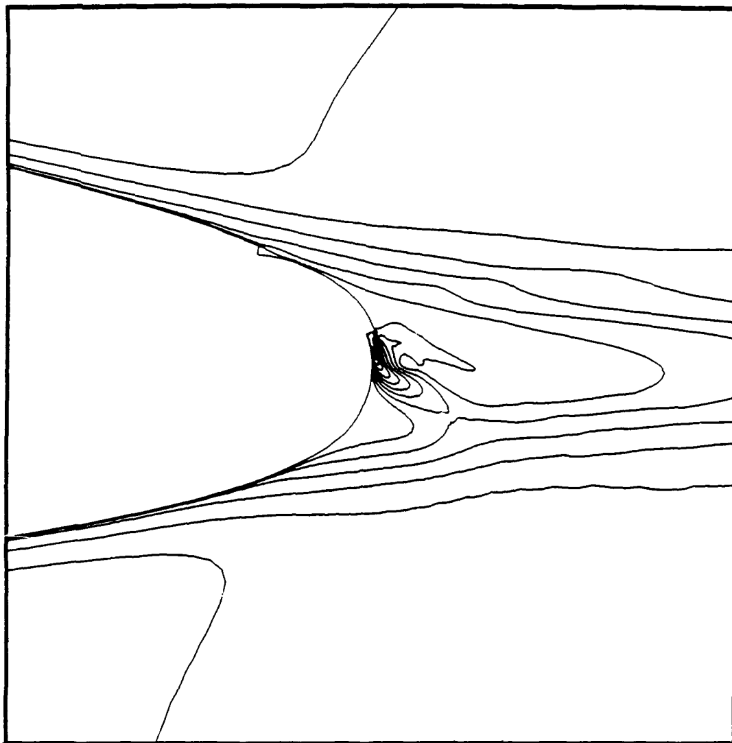
Figure 21. Case AB Mach Contour - Trailing Edge
