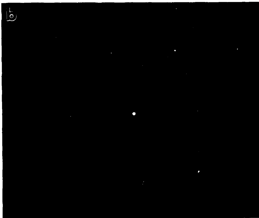
Figure 8. (a) Polycrystalline \gamma segregate, (b) diffraction pattern showing a [101]_{\gamma} zone.
