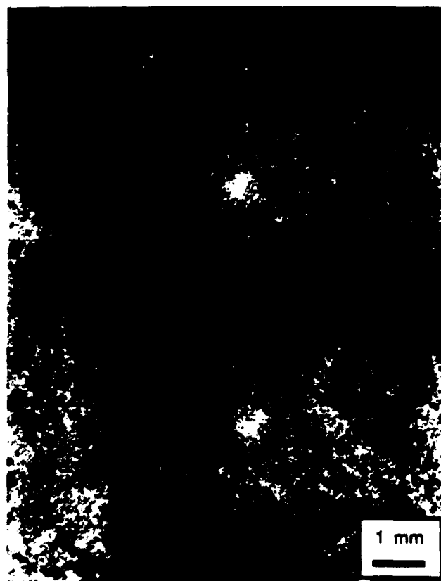
Fig. 14—Optical micrograph of a cross section of a sample infiltrated by aluminum followed by lead. Dark regions are lead or fiber, and light regions are aluminum. Infiltration occurred upward. Infiltration parameters were V_f = 0.23 , 99.9 pct pure Al, T_f = 608 K, T_0 = 993 K, \Delta P_f = 3.5 MPa; sample diameter was 11 mm.
