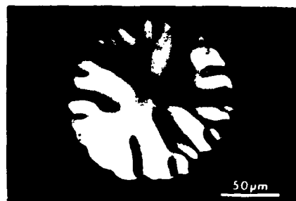
Figure 15 A large buckled blister in a coating in the process of undergoing delamination, viewed with the Nomarski interference contrast mode of microscopy. The outer ring surrounding the buckled centre is the zone in which radial slippage occurs to relieve the radial stress.
