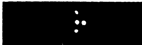
Figure 5. Pattern of Four Spots on the P-1 Phosphor Screen when the \text{LaB}_6 was irradiated at 248 nm. Spot diameter \approx 1.45 mm. (Note: One of the five holes was occluded).
