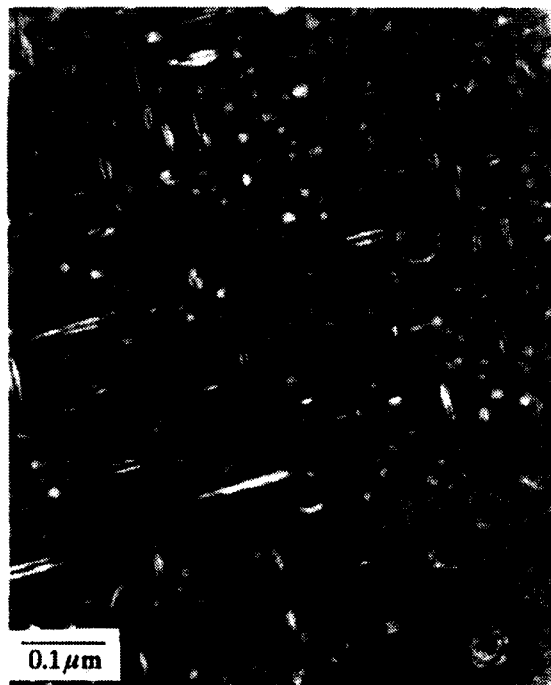
Figure 6. Superlattice dark field image of 2090 matrix revealing \delta' , \beta'/\delta' , \theta' , and \text{T}_1 precipitates.
