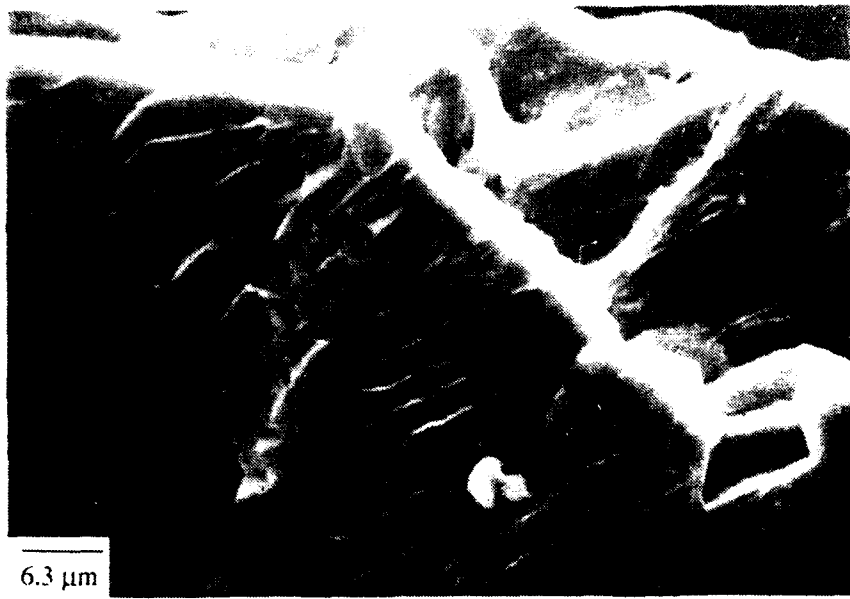
Figure 11. SEM micrograph of shear bands on fracture surface.
