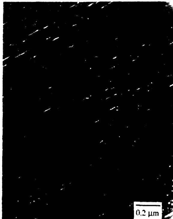
Figure 8. Dark field image using \delta'/\theta' superlattice reflection.
