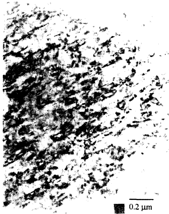
Figure 7. Bright field image showing T_1 and \theta' plates.
