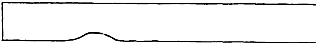
Figure 8.3: Overview of new asymmetrically constricted channel
