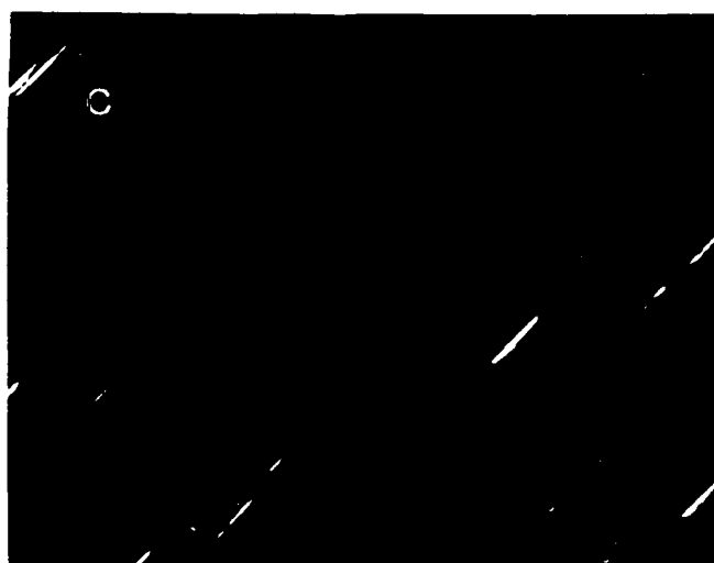
Figure 4.1 Darkfield TEM photographs, Z=100 , showing distribution of S' in a) 8090 stretched 6% b) 8090 unstretched c) 8090 duplex aged (continued next page).
