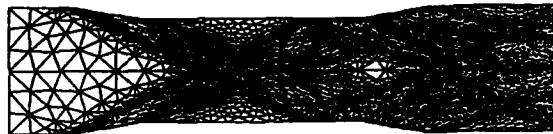
(c) Mesh: 5714 elements, 3005 nodes
