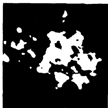
e) Aggregate: (513X) 54.2 \mu\text{m} X 52.4 \mu\text{m} 1.12 g/cc
