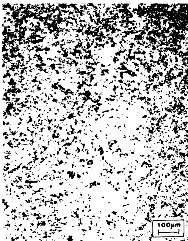
Figure 2. CF6-80C2 5th Stage LPT Blade: As-Cast Oversized Blade and Fully Machined Blade and Representative Microstructure After HIP (2300°F/4h/25 KSI) and Heat Treatment (1650°F/16h).
