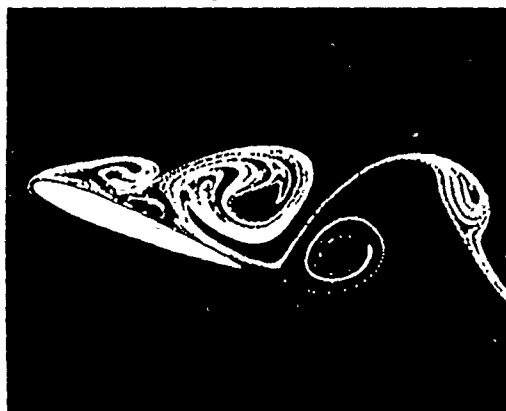
Fig. 16. Instantaneous pattern of the velocity vectors for the separated flow over an NACA-0012 at high angle of attack \alpha = 20^\circ . Navier-Stokes solution from [16].
