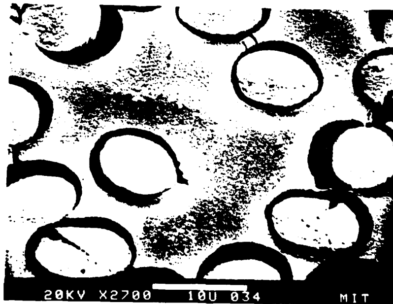
Figure 14: SEM micrograph showing crevices along the perimeters of graphite fibers in a planar G/6061-T6 Al MMC six-ply plate electrode that was anodically polarized at 2.0 \text{ V}_{\text{SCE}} for 3.2 h in deaerated 0.5 \text{ M Na}_2\text{SO}_4 of pH 7 at 30^\circ\text{C} . The formation of crevices was caused by \text{CO}_2 evolution, resulting from the oxidation of graphite.
