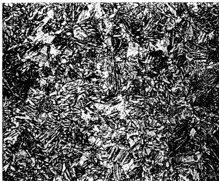
D. ROOT CORE MICROSTRUCTURE: LATH MARTENSITE, HRC 26, 500X
