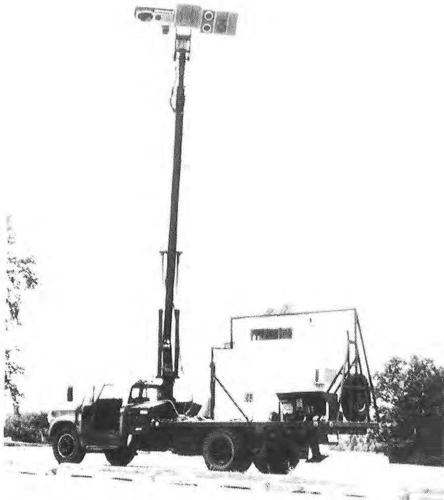
Fig. 1 Photograph of the Millimeter-Wave Polarimeter system with the boom extended about half way.
