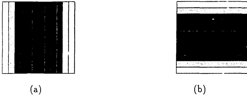
Figure 6: The transmission masks for modulating the intensity of a focus spot based on its displacement from the optic axis along the (a) x axis or (b) y axis.
