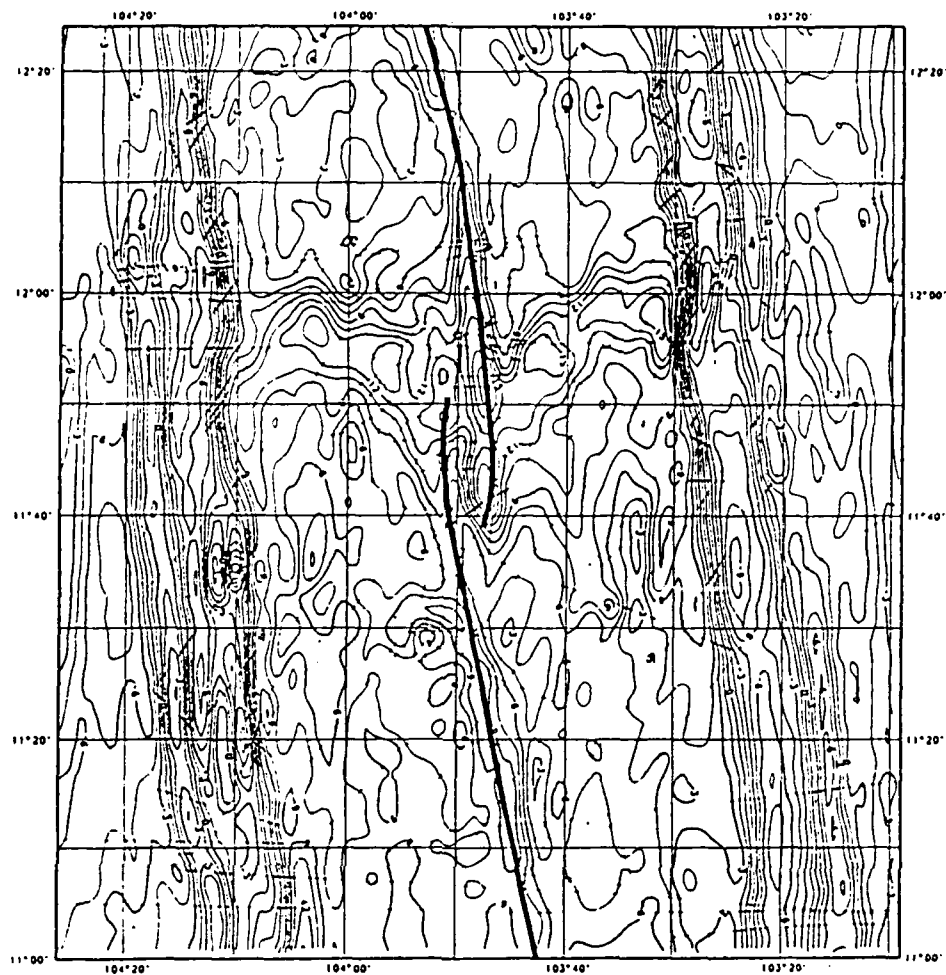
Figure 1. Inversion solution (from 1 km grid) as described in text. The contour interval is 1.5 A/m and ticks on contour lines show track coverage.
