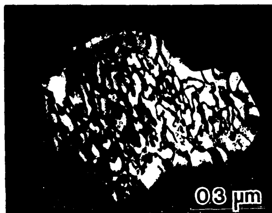
Fig. 5. Dark field image of the DO_{19} phase using a superlattice reflection. The fine antiphase domains can be seen.
